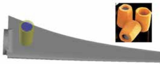
Fig. 3. In direct pour filling, the metal is poured through a ceramic filter directly into the mold cavity via pouring cups (shown in inset).
